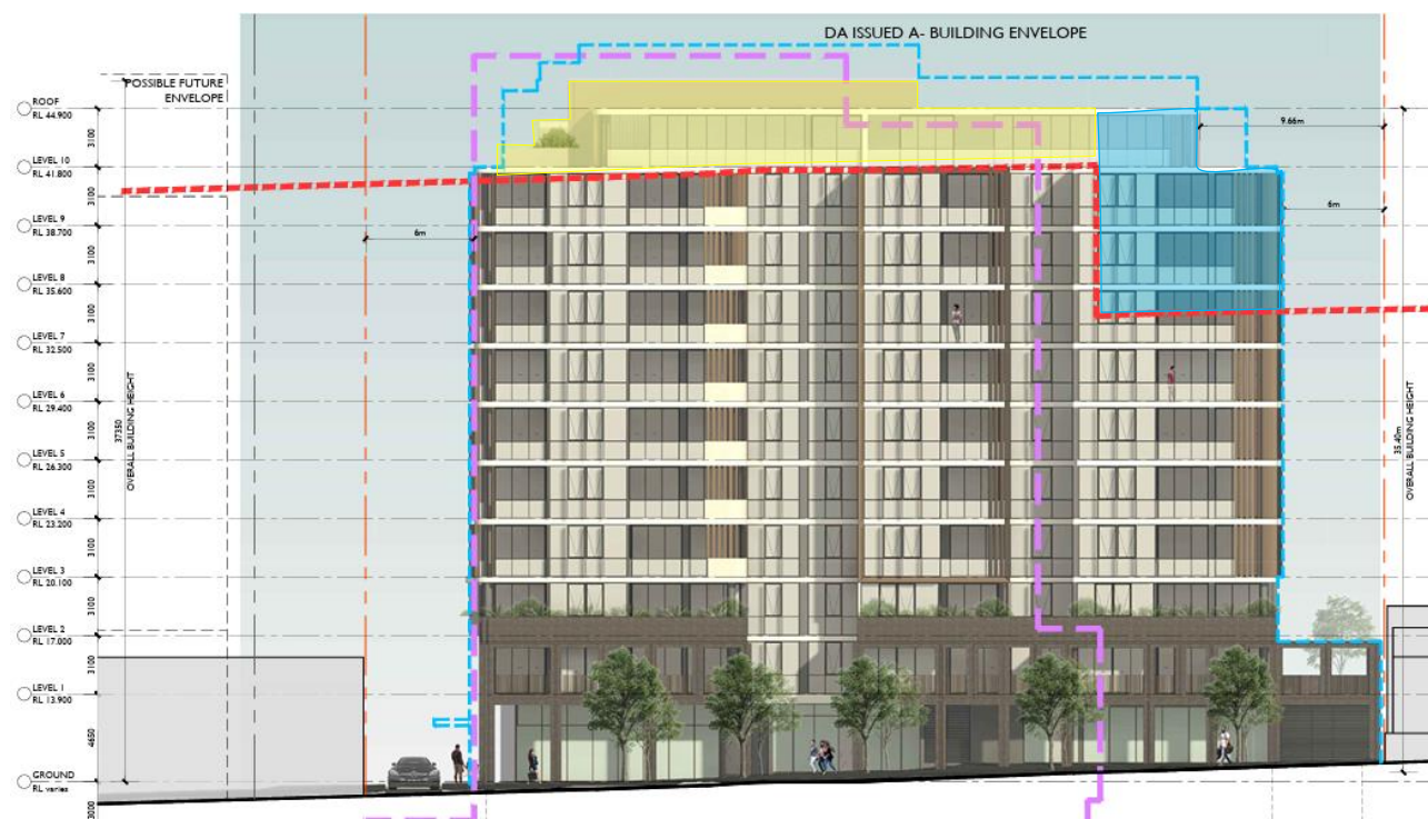
Figure 2: Excerpt from Eastern Elevation Plan (A-201 Issue C by ADM Architects) illustrating extent of variation to permitted maximum building height controls of 32m (in yellow) and 24m (in blue). The blue dotted line depicts the building envelope of the previously submitted plans for this Development Application (Issue A). The pink dotted line depicts the building envelope of the previously approved valid development application.
